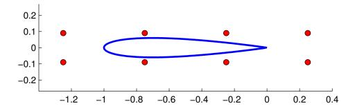
Figure 1: Airfoil surface and deformation control nodes
