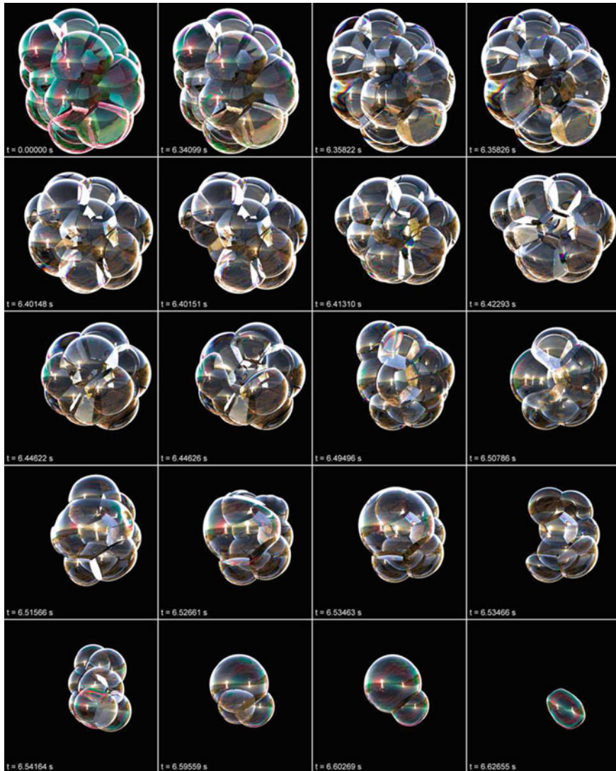
Fig. 10 Collapse of a foam cluster, visualized with thin-film interference taken from [29]
