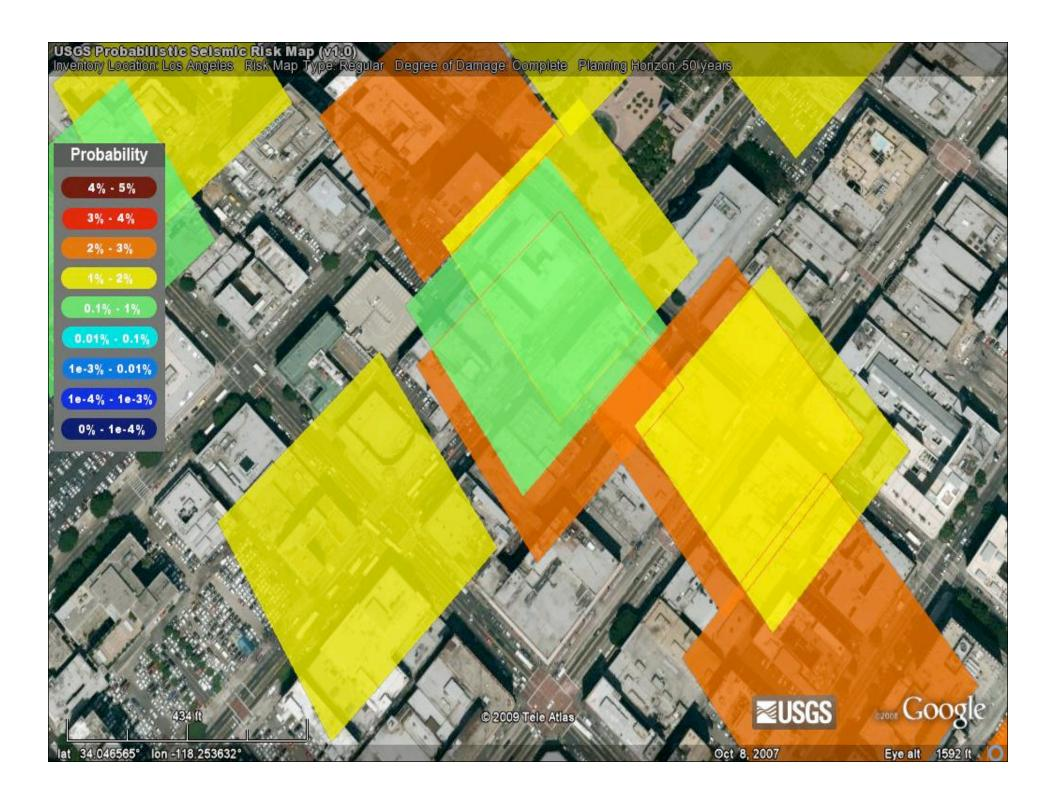
USGS Probabilistic Seismic Risk Map (v1.0) Building Type: C1L Seismic Design Level: Low-Code Degree of Damage: Slight Planning Horizon: 50 years
